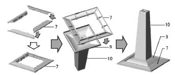
**Note:** The additional base (7) is designed to fasten the street lamp more securely. If the street lamp is installed on a flat ground and there is no external force (such as high wind or man-made interference), or if the street lamp is used outdoors and it can be fixed on the ground by fastening ground nails; there is no need to install additional base (7). In other words, users can decide whether to install the additional base (7) according to the actual condition.
